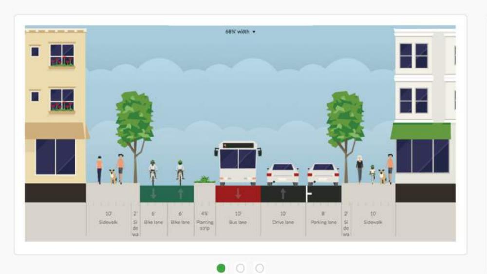
Polk Street is wide enough to accommodate a separated 2-way cycle track on one side of the street and to retain
