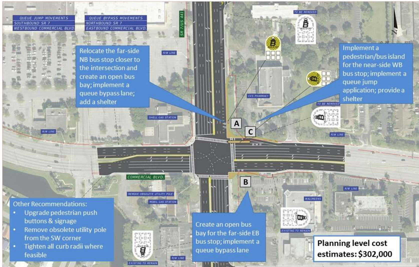
Figure 5: Recommended Improvements at SR 7 & Commercial Blvd
