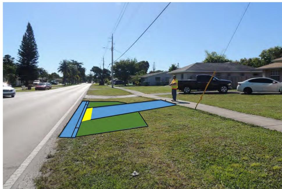
Figure 225.2.1 Accessible Boarding and Alighting Area for Flush Shoulder Roadways with Connection to Sidewalk
