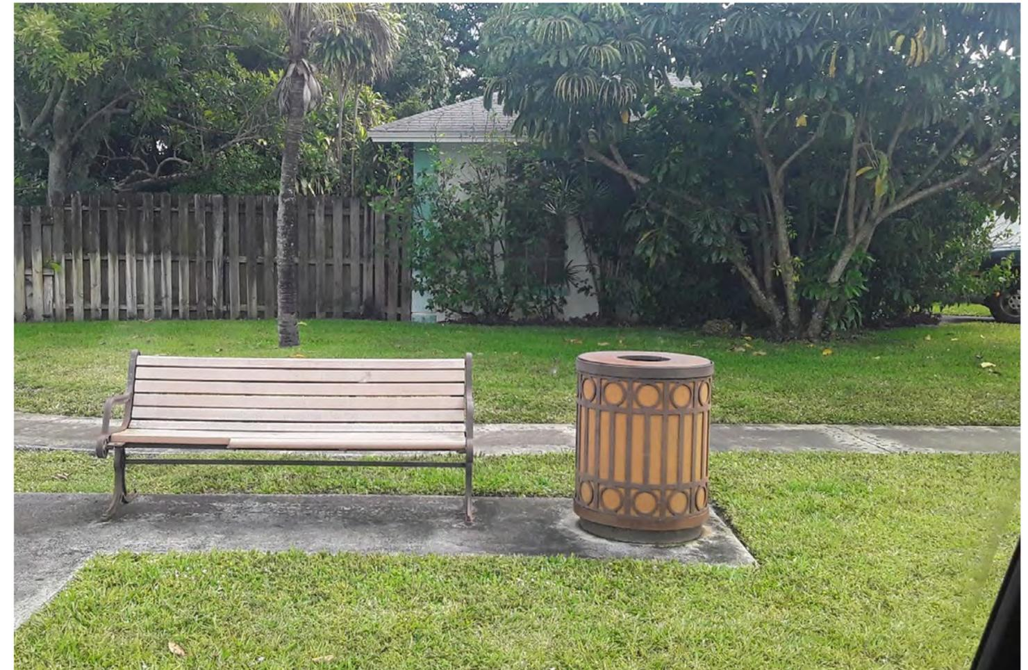
Shuttle stop at NW 55th Ave. and NW 17th Ct, which is not ADA accessible due to: lack of sidewalk connection between the bus stop and sidewalk, no wheelchair waiting area, or signage.
