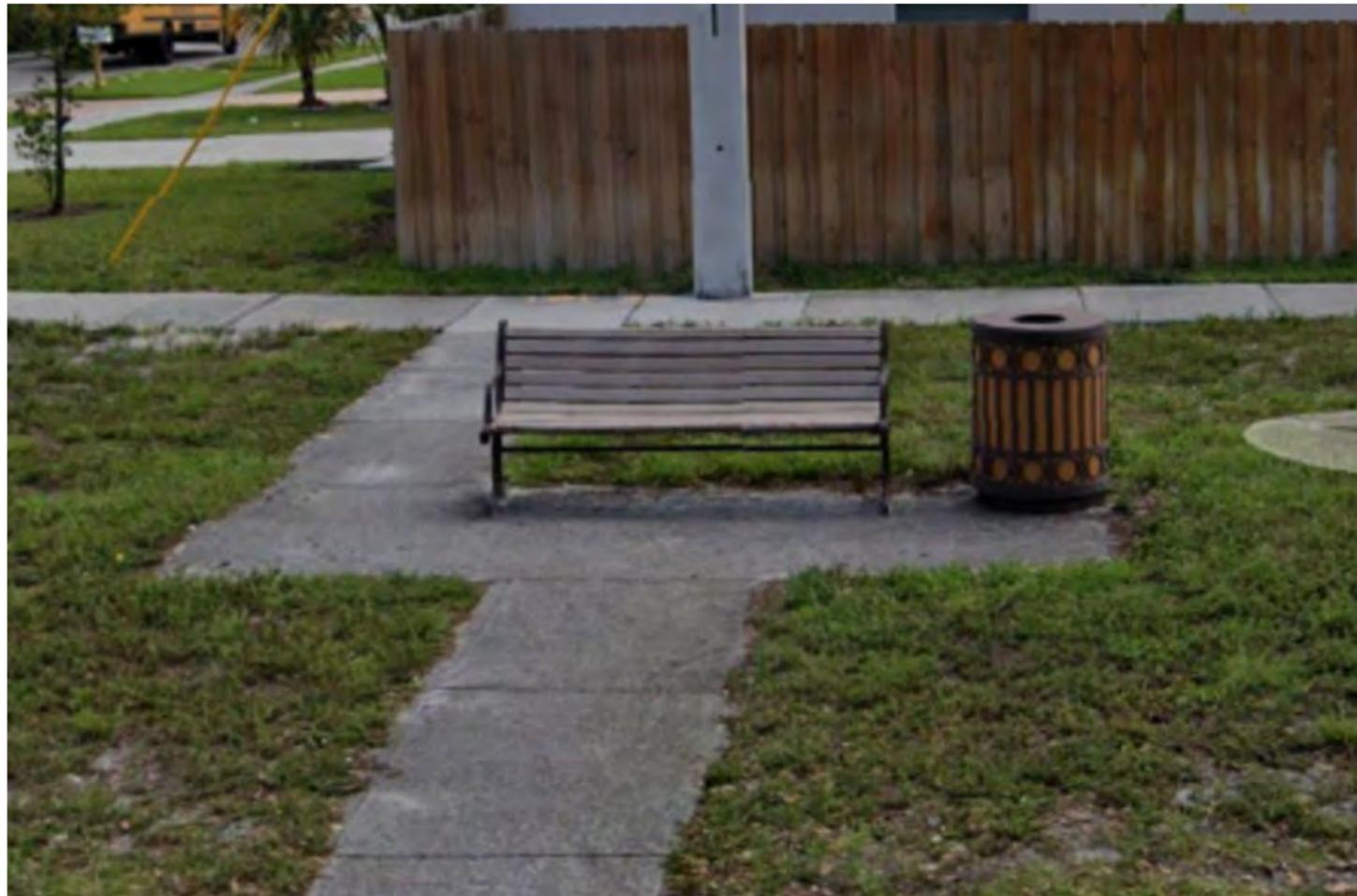
Shuttle stop at NW 55th Ave. and NW 19th St. No wheelchair waiting zone or detectable warning strip, nor is there signage to indicate it's a bus stop.
