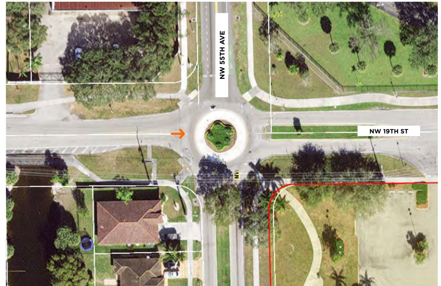
Existing 19th St. and NW 61st Ave roundabout overlaid on the 19th St. and 55th Ave. intersection and reduced in size by about 20% to accommodate existing curb lines and ROW.
