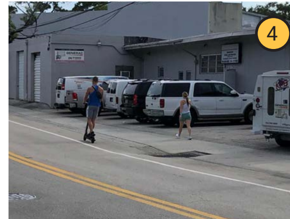
4 At-grade sidewalk directly abuts back-out parking. Scooter in bike lane.
