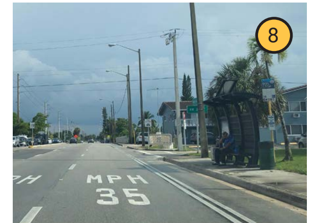
8 Pavement markings and signage to alert drivers of 35 MPH speed limit. The only BCT stops with shelters and benches are those closest to Oakland Park Blvd.
