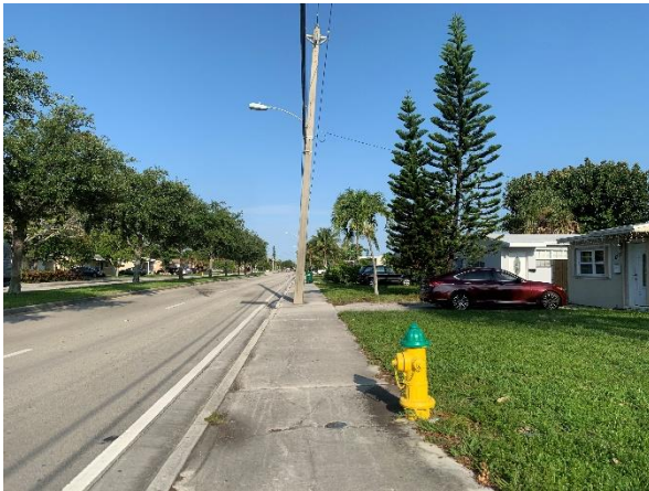
Street fixtures are within the sidewalk, which prevents a clear pedestrian zone.
