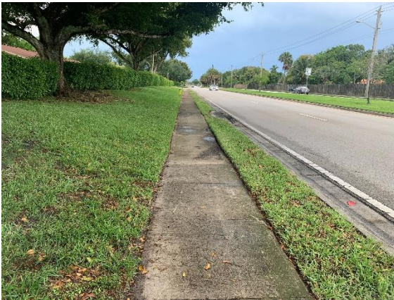
Sidewalk on the north side of Southgate Boulevard with a buffer between the sidewalk and curb, also known as a furnishing zone.
