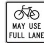
Use of R4-11 Sign on Roads with Speed Limits Above 35mph
